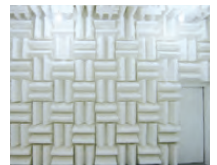
Research laboratory: anechoic room with PET sound absorbing wedges
