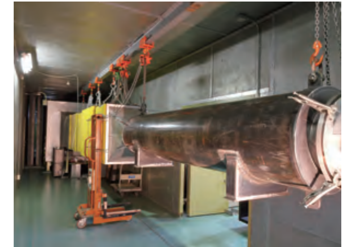
Noise control for Vessel "LINEAR SILENCER" for engine exhaust gas(State of the performance test)
