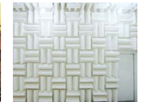
Research laboratory: anechoic room with PET sound absorbing wedges
