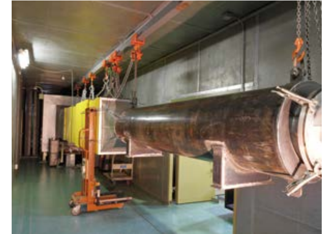
Noise control for Vessel Silencer for engine exhaust gas(State of the performance test)
